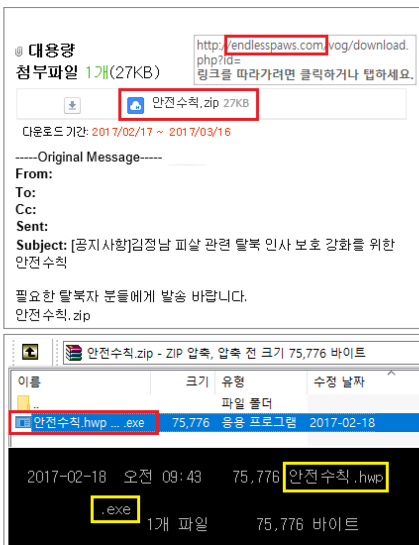
[Figure 8] Distributing the malware by disguising as the safety guideline
